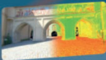
An integrated auto-adjusting high-resolution camera delivers «photo-realistic» images that can be applied to point clouds to enhance interpretation and documentation.
