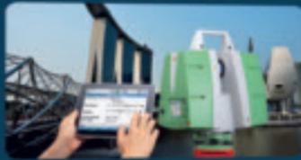
With integrated WiFi, Leica ScanStation P20 can be remotely controlled by a Leica CS10/CS15 field controller or by an iPad, iPhone or similar Smartphone. Remote control ensures comfortable and safe use when the scanner is in a restricted environment and allows convenient display viewing.
